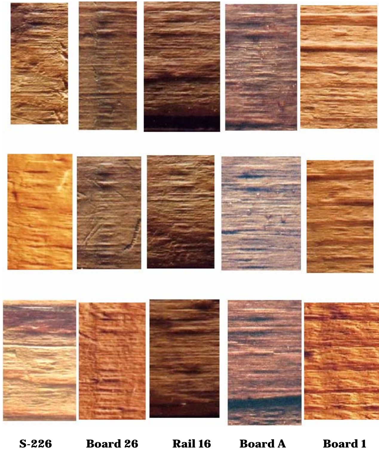
Figure 33: Samples of some of the clearest examples of the inner defect series on the boards. The boards vary in condition and shrinkage. Board 1 has the most deterioration, and Board s-226 appears worn, with little detail in this area. The photos vary in lighting and quality. While the author was careful to adjust all of the images to the same scale, some slight variations may occur.
